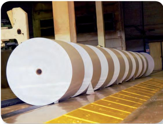
The company mastered the production of low-weight newsprint (40 g/m<sup>2</sup>) in 2017, which had not been previously produced by any Russian manufacturer. The advantage of these products is the increased area of the paper web in one roll, which allows to print more products from 1 ton of paper.
