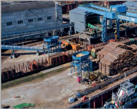
**in 2016, the company launched a new automated line for unloading and transporting wood raw materials, which consists of a receiving storage hopper and belt conveyors that feed commercial wood chips to cumulus storage, ensuring that they are mixed with the process wood chips produced in the company. This made it possible to improve the quality of raw materials entering the thermomechanical material shop.**
