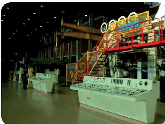
In 1994, the Voith company (Germany) launched the highspeed papermaking machine No. 8, designed at the most modern technical level. Its operating speed is 1300 meters per minute, and its capacity is 250,000 tons of production per year.
